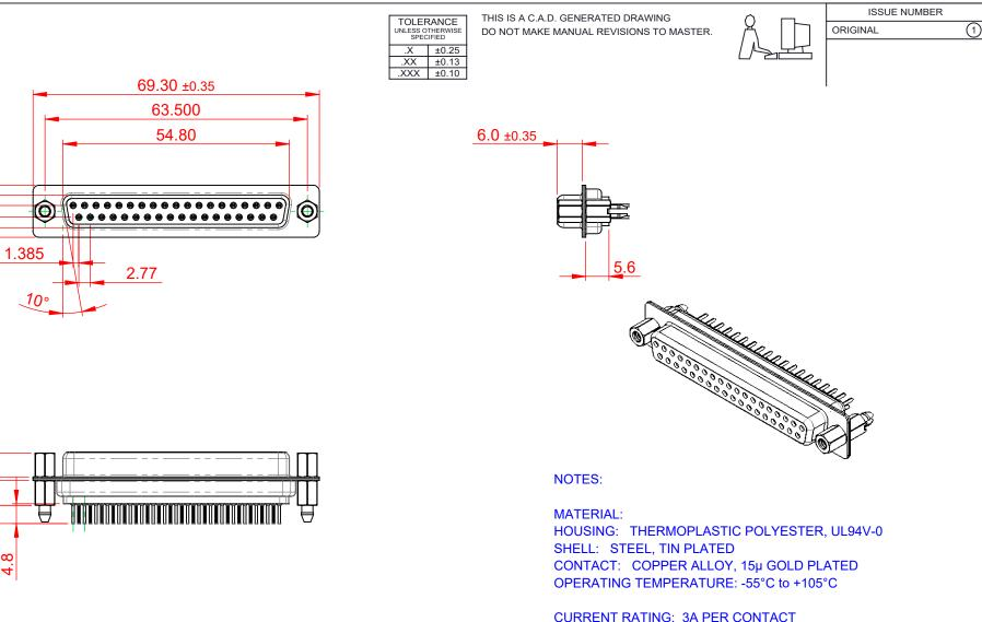
CURRENT RATING: 3A PER CONTACT CONTACT RESISTANCE:  $25m\Omega$  MAX. INSULATOR RESISTANCE:  $5000M\Omega$  min. DIELECTRIC WITHSTANDING VOLTAGE: 1000V AC rms
