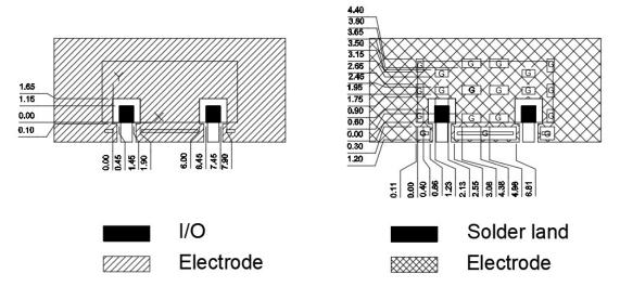
3.6 The recommended shielding case layout guide (min)
