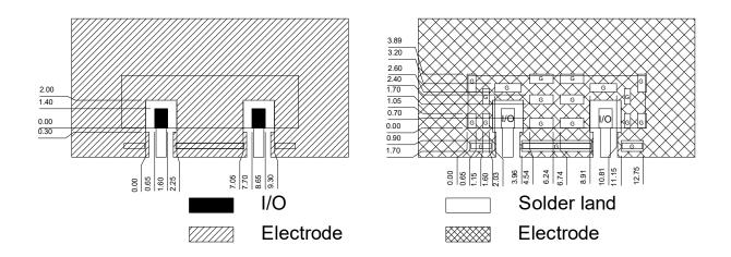
The recommended shielding case layout guide (min)
