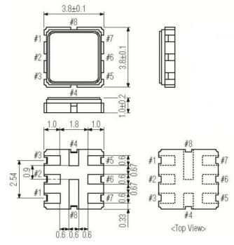
**Pin Connections** \* In/Out #1 #2 Ground Ground #3 #4 Ground \* Out/In #5 Ground #6 Ground #7 Ground #8 \* Filter is symmetrical
