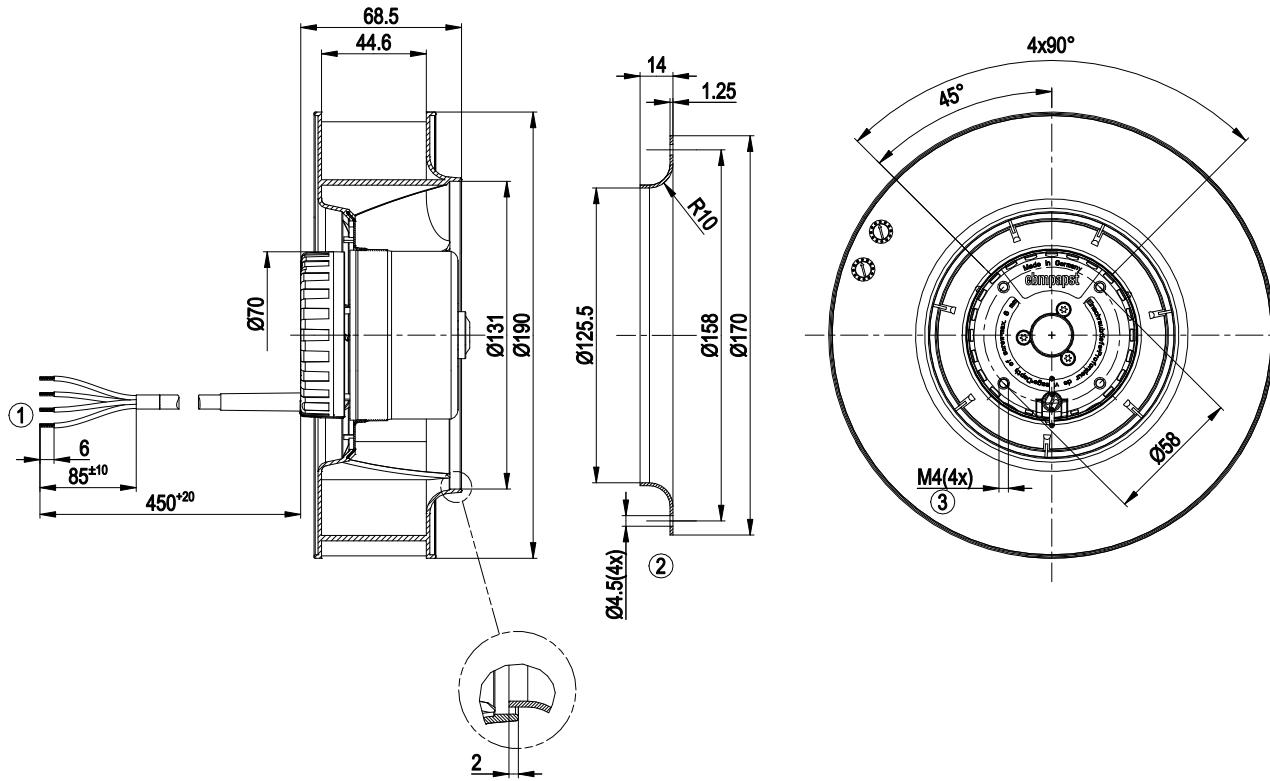
1 Cable AWG20 4x 0.5 mm<sup>2</sup>, 4x crimped splices
