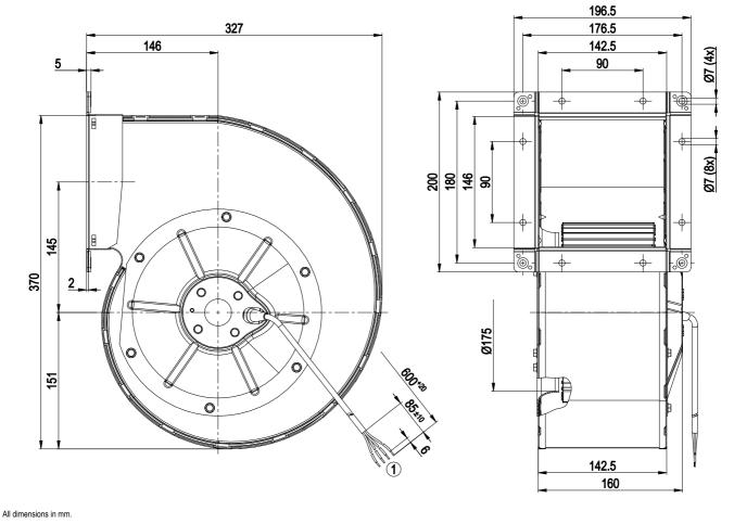
Cable silicone 4G 0.5 mm<sup>2</sup>, 4x crimped splices
