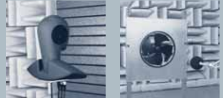
Room for precision noise measuring
