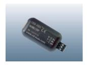
Part Number: 21490-1-0174 The ebm-papst USB RS485 adapter connects RS485 devices to a computer USB. This also requires the ebm-papst EC Control software version 2.0 or later. The USB drivers required for operating the adapter are also included.
