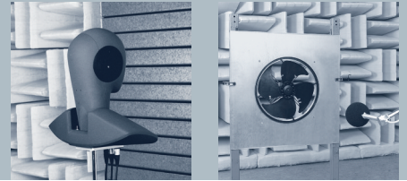
Room for precision noise measuring
