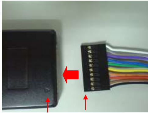
Figure 2-8: Plugging the Wire Harness into the Analyzer
