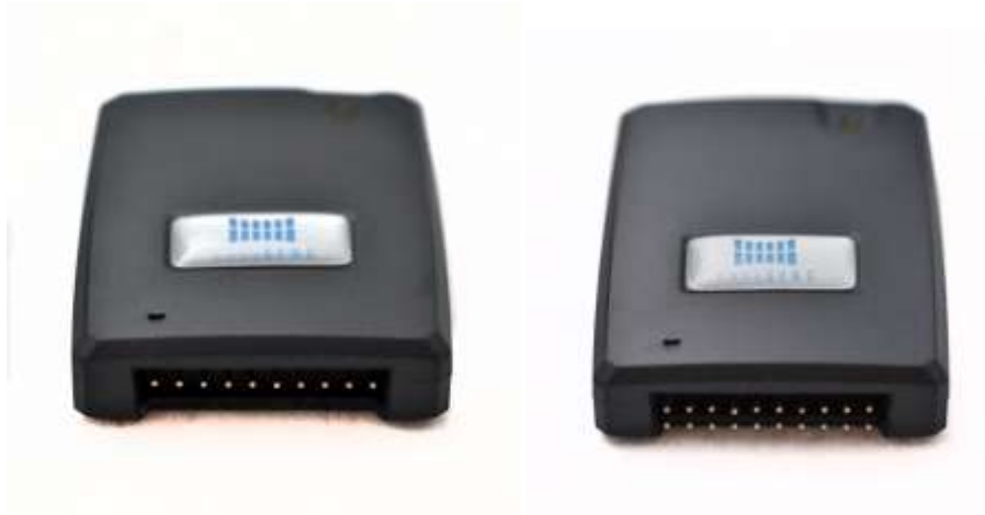
Figure 1-4: Front Panel showing the ES-DLA-8 and ES-DLA-16 Logic Probe Connectors
