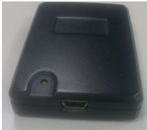
Figure 1-3: Rear Panel showing the USB Connector
