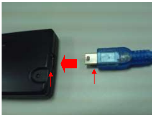
Figure 2-6: Connect the USB Cable to the Logic Analyzer
