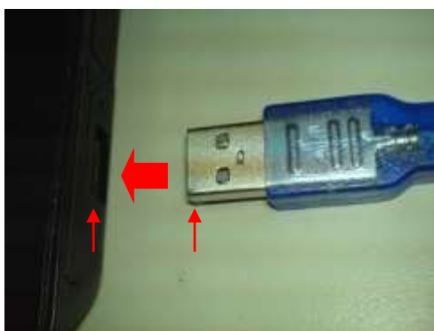
Figure 2-7: Connect the USB Cable to the Computer
