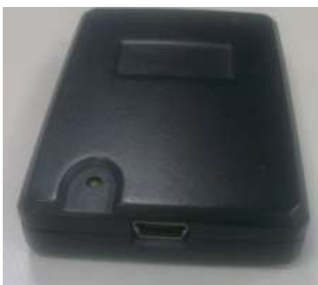
Figure 1-3: Rear Panel showing the USB Connector
