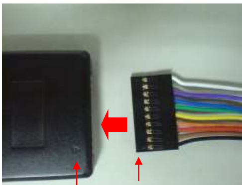
Figure 2-8: Plugging the Wire Harness into the Analyzer
