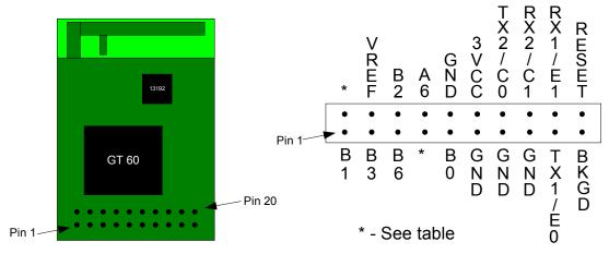
Top View (Interface Header on bottom of PCB)
