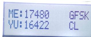
6.4.2 Press and hold Button 3. While holding Button 3, press and release RESET. Continue to hold Button 3 until you hear a beep. Release Button 3 and the system will be transmitting at 2.4GHz on the internal chip antenna with GFSK modulation.
