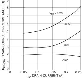
Fig. 6 Drain-Source On-Resistance vs. Drain-Current
