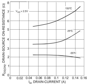
Fig. 5 Drain-Source On-Resistance vs. Drain-Current
