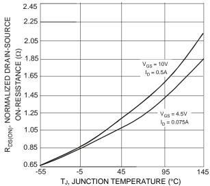
Fig. 3 Drain-Source On-Resistance vs. Junction Temperature
