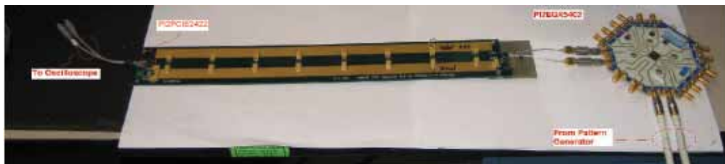
Figure 6: the test set-up for the PI2PCIE2422 eye test
