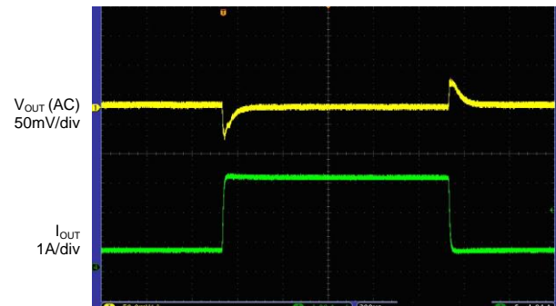
Load Transient Response ( V_{IN}=3.3V , V_{OUT}=2.5V , I_{OUT}=0.5A to 3A )
