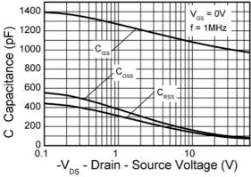
Capacitance v Drain-Source Voltage
