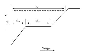
Basic gate charge waveform
