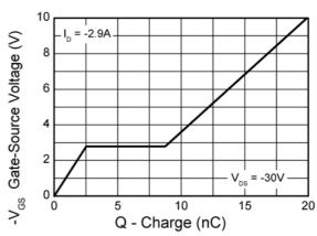
Gate-Source Voltage v Gate Charge
