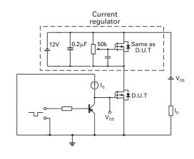
**Gate charge test circuit**
