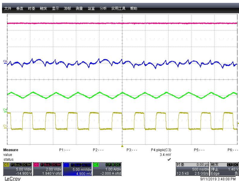
Figure 9. Output Voltage Ripple, I_{OUT} = 1A ( V_{OUT} = 1.8V )
