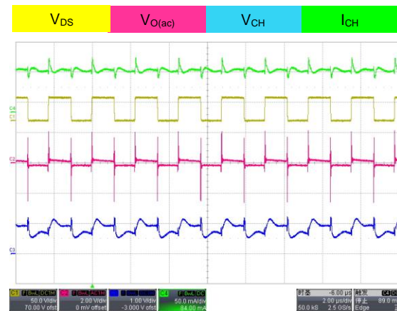
PWM to Analog Dimming ( f_{PWA}=10\text{ kHz} , 50% Duty)
