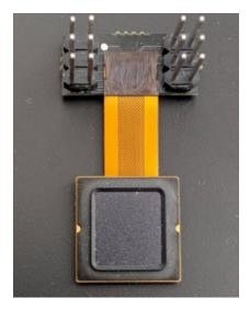
Showing how the BM-Lite Flex Cable should be mounted on the FPC5924 board.
