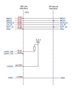
Example schematic of BM-Lite interface using SPI
