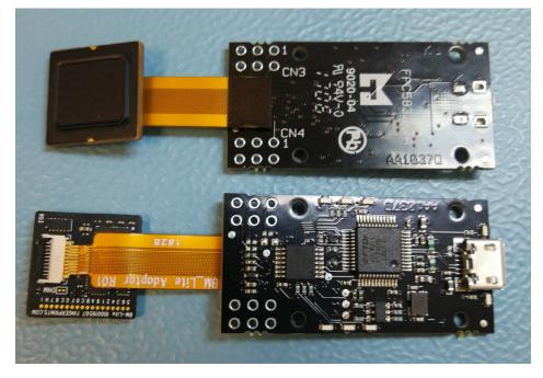
The FPC5832 is an USB-SPI adapter using an FTDI FT232H converter. The CN3 connector is pincompatible with CN2 on FPC5924, and CN4 is pin-compatible with CN3 on FPC5924.
