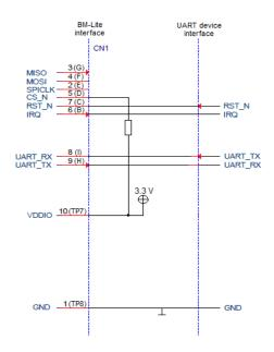
Schematic of BM-Lite interface using UART
