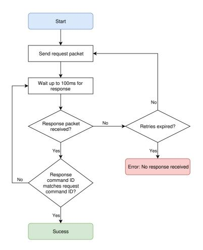
The values used for timeout or number of retries should be tuned to the specific application.
