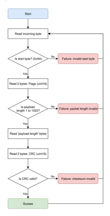
If the packet length or checksum is invalid then it is technically more correct to roll the incoming stream back to when the start byte was found. However in practice this has little appreciable impact.
