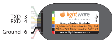
Figure 6 :: Serial interface connections
