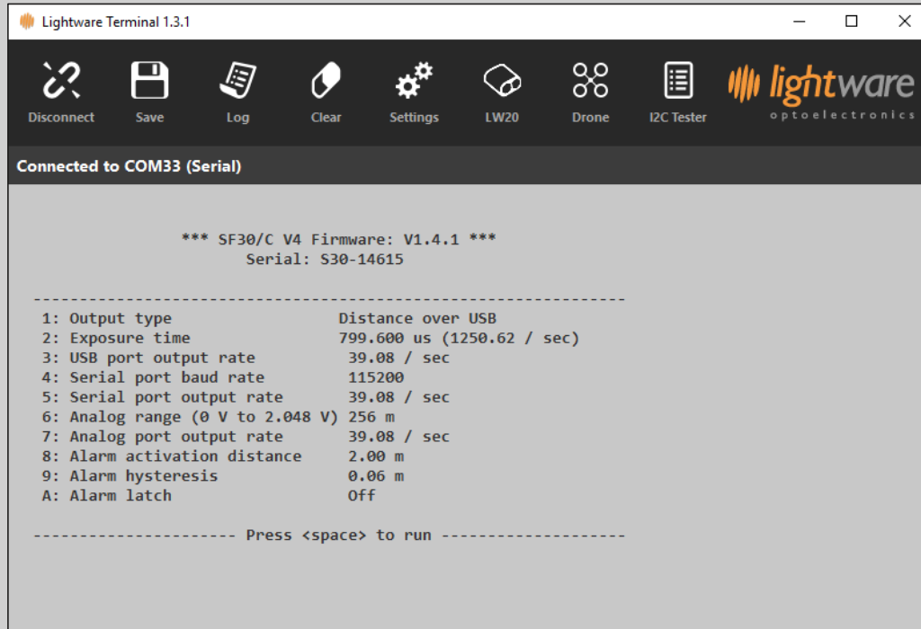
Figure 2 :: LightWare Terminal showing menu options
