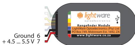
Figure 4 :: Regulated +5 V DC power supply connections
