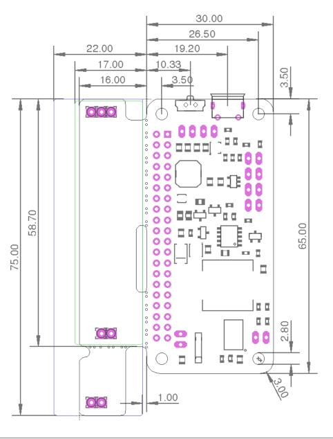
Note that this drawing is a view of the component side or bottom of the PCB.
