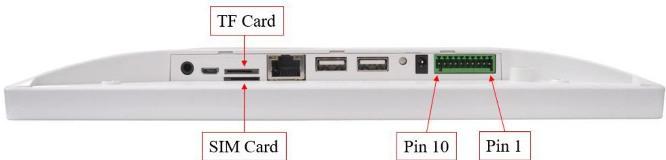
Figure 5: TF card slot, SIM card slot and RS232+RS485+Relay connector
