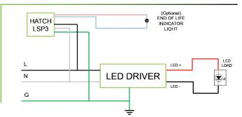
**EOL Indicator:** When illuminated, LSP3 is working correctly. When the indicator goes out, LSP3 needs to be replaced as soon as possible.
