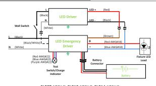
For additional wiring diagrams please visit https://www.hatchlighting.com/elp-alternate-wiring-diagrams
