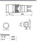
Recommended hole size for installation: Ø12mm
