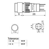
Recommended hole size for installation: Ø12mm
