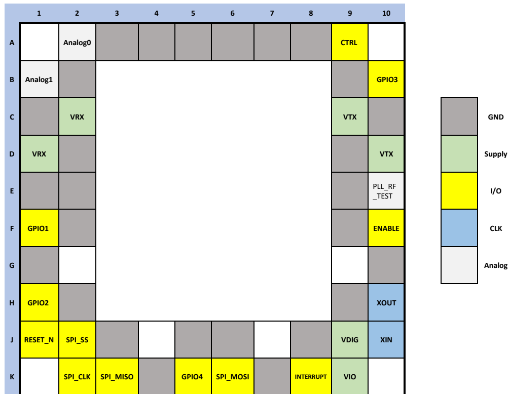
Figure 3.1. Pin configuration of the A121 sensor, top view.
