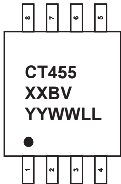
Figure 24: CT455 Device Marking for Eight-Lead SOIC Package
