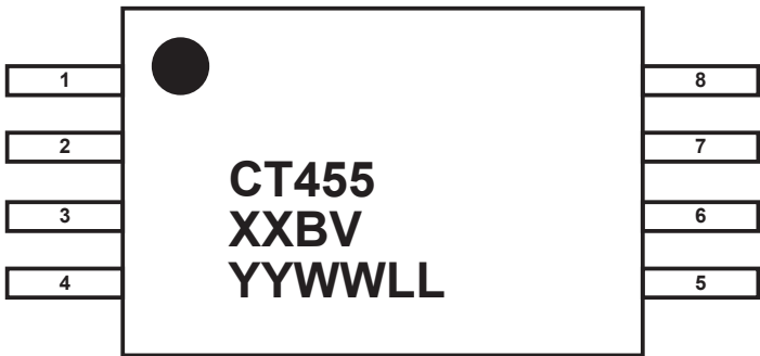
Figure 23: CT455 Device Marking for Eight-Lead TSSOP Package
