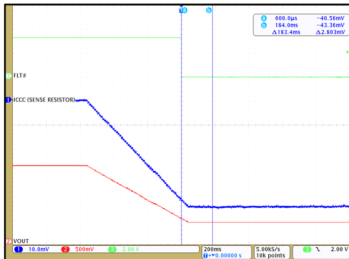
Figure 15. CT431 OCD enabled at -110% of -50 A PK and FLT# is LOW
