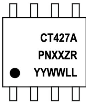
Figure 24: CT427 Device Marking for 8-lead Package
