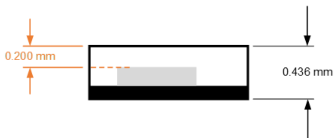
Figure 36: XtremeSense TMR Sensor Location in z Dimension for CT815x in 4-lead LGA Package
