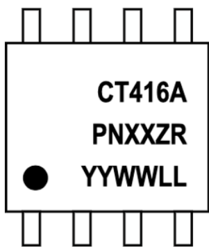
Figure 44: CT416 Device Marking for 8-lead Package
