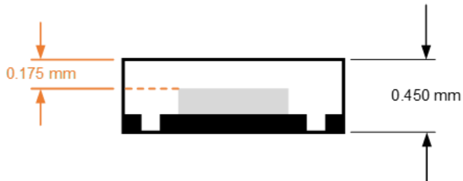
Figure 15: XtremeSense TMR Sensor Location in z Dimension for CT100 in DFN-6 Package
