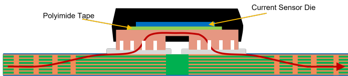
Figure 5: No Vias Under Copper Pads Example
