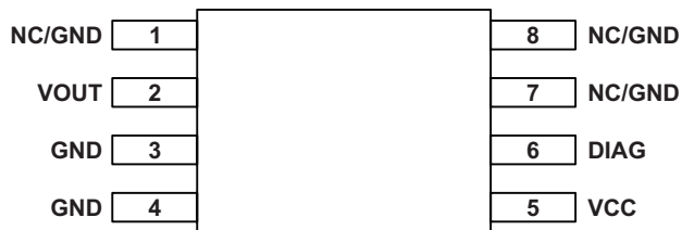
Package LE, 8-Pin eTSSOP Pinouts
