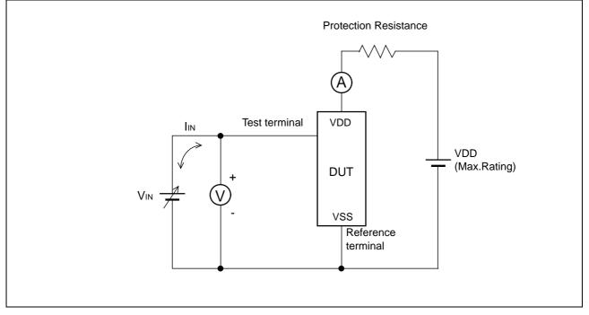
Note : The voltage V<sub>IN</sub> is increased gradually and the current I<sub>IN</sub> of 300 mA at maximum shall flow. Confirm the latch up does not occur under I<sub>IN</sub> = ± 300 mA. In case the specific requirement is specified for I/O and I<sub>IN</sub> cannot be 300 mA, the voltage shall be increased to the level that meets the specific requirement.
