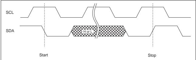
Note : At the write operation, the FRAM device does not need the programming wait time (twc) after issuing the Stop Condition.
