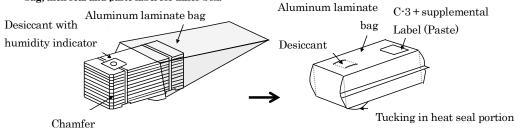
(4) Put the aluminum laminate in inner-holder, store in inner box.
