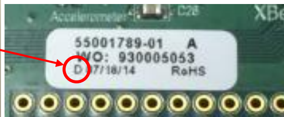
Image 3: Notation of Revision Level on Label
