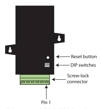
The adapter is switch-selectable between RS-422 half duplex/full duplex, and RS-485 modes (see DIP switches on page 24). The function for several pins varies between RS-422 and RS-485 modes.
