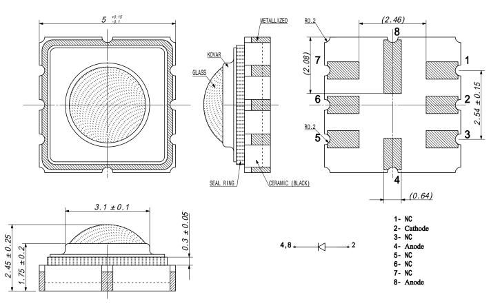
Recommended Soldering Pattern [mm]
