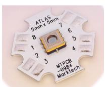
Aluminum Core Board 0.040" (1.02mm) Thickness Overall Board Dimensions: +/- 0.010" (0.254mm)
