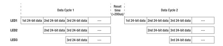
The single wire data transfer protocol supports 24-bit data for each LED RGB display data refresh. THE IC receives 24-bit data and passes the remaining data to next LED. The 24-bit data consist of red, green and blue data, each with 8-bit width, and are transferred with MSB first.
