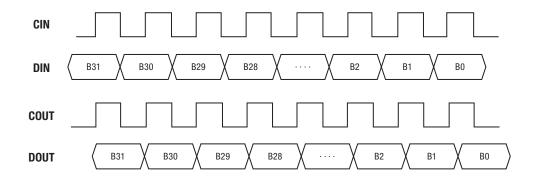
The serial command is transmitted with MSB first, DIN is latched at the rising edge of CIN clock. COUT and DOUT are re-generated for the next RGB LED. COUT is inverted from CIN. When 32 consecutive 0's are encountered, the next 1 is expected to start a 32-bit command, i.e., FLAG[2:0]=111. When FLAG[2:0]=111, then DIMMING, BLUE, GREEN and RED fields are latched respectively.
