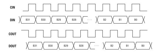
The serial command is transmitted with MSB first, DIN is latched at the rising edge of CIN clock. COUT and DOUT are re-generated for the next RGB LED. COUT is inverted from CIN. When 32 consecutive 0's are encountered, the next 1 is expected to start a 32-bit command, i.e., FLAG[2:0]=111. When FLAG[2:0]=111, then DIMMING, GREEN, BLUE and RED fields are latched respectively.
