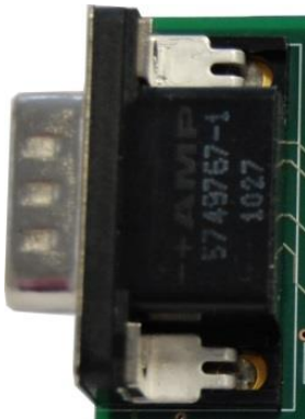
Figure 2.3: 15-pin VGA connector for power supply
