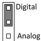
Figure 2.13: Jumper settings for analog/digital enable
