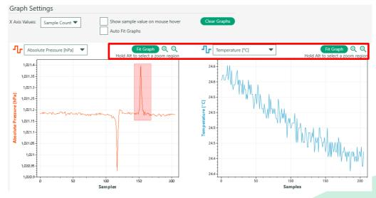
• **Graph Selection:** there are two graphs being presented simultaneously. The user can use the drop down menus with three options to choose which signal to display in each plot.
