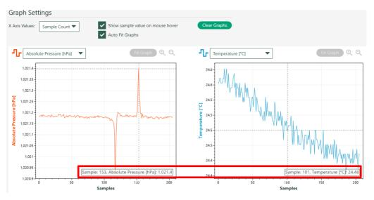
• **Auto Fit Graphs:** when deactivated, the functions Fit Graph, Zoom In, and Zoom Out will become enabled. Move the cursor to the graphs and, while holding Alt, click and drag the mouse to create a zoom region to zoom into and check sensor performance in detail. To zoom out click the Fit Graph icon.
