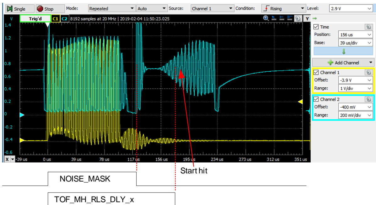
Figure 6: Typical send and receive signals
