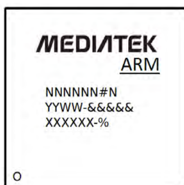
Figure 7-1 Device Top Marking
